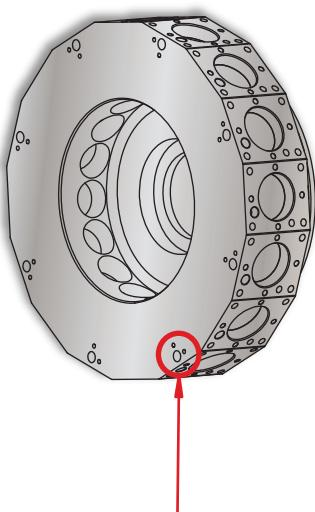
Capto mechanism access through turret face
