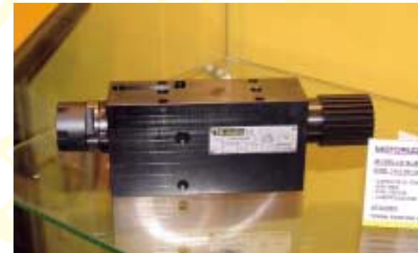
Driven unit to DECO 20/26
